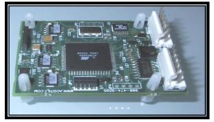
SOLID STATE High Accuracy advanced Pitch / Roll / Temperature compensated COMPASS / MAGNETOMETER system is built around a state of the art CMOS microcontroller utilizing AOSI's proprietary algorithm on a 1.5" x 2" assembled PCB with a total height including tilt sensing elements of less than 0.5".
